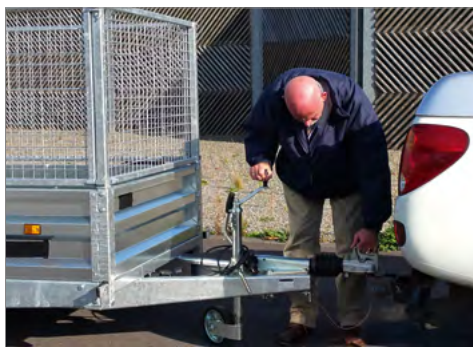
Figure 18. Coupling a trailer
